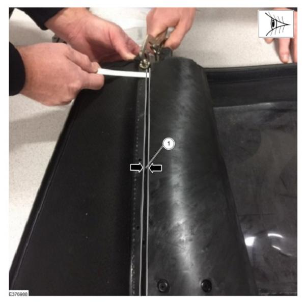
**11.** Drill the holes using a 5 mm drill bit. Starting at the bottom and working toward the top. Do not drill into the surrounding stitches. Remove the clamps once all 5 holes have been drilled. (Figure 7)
