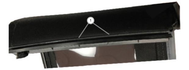
**15.** Carefully clean the rear window assembly removing all metal shavings.
