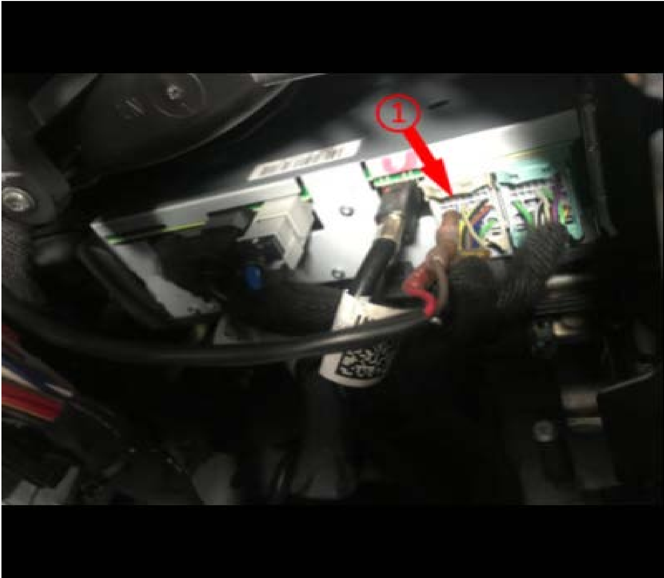
Disconnect the gray A11 Radio X2 Connector (1).
