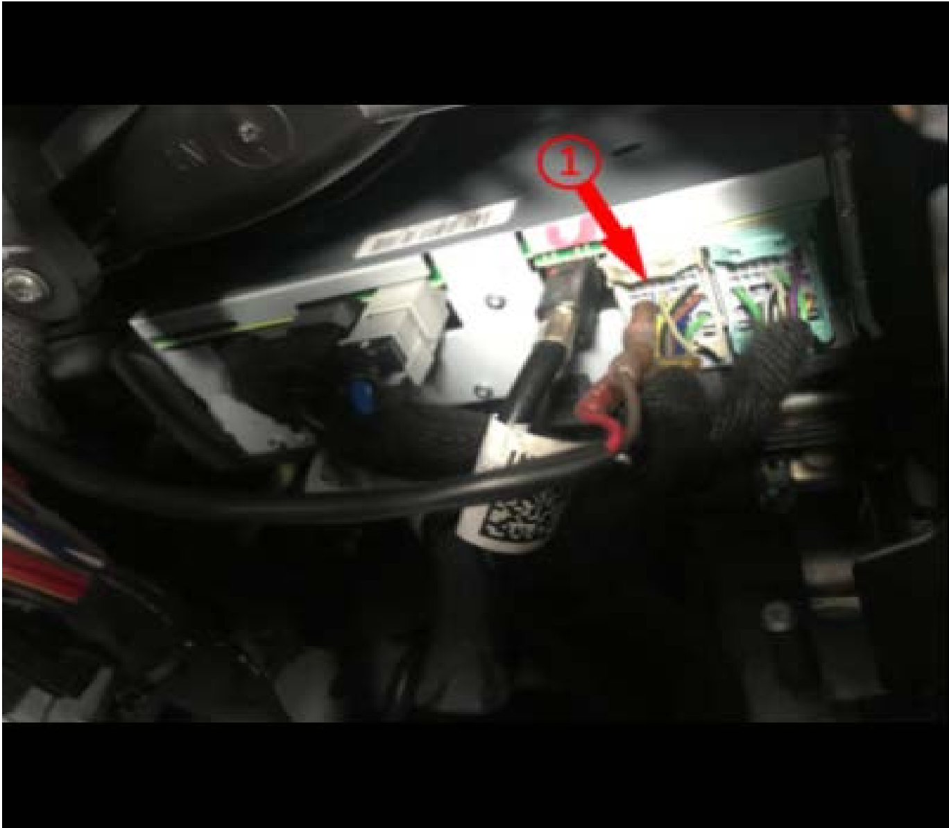
Disconnect the gray A11 Radio X2 Connector (1).
