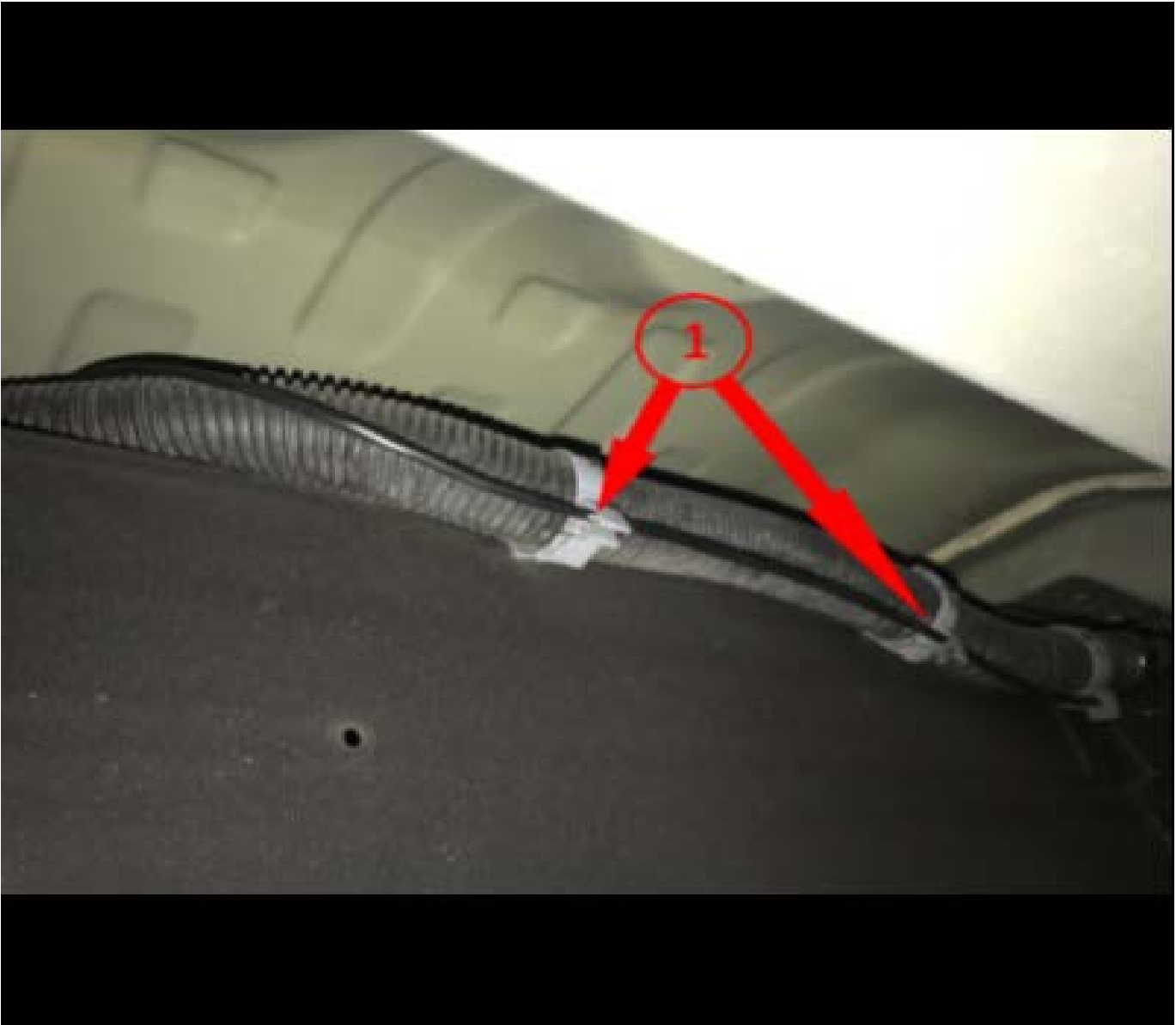
Utilizing the harness clips (1) or zipties to secure the data cable along the harness.
