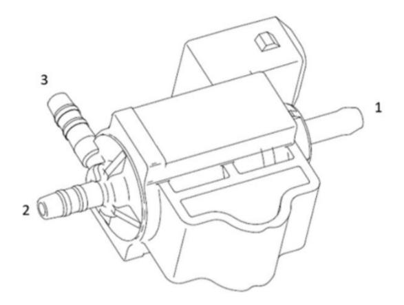
Note: Check port #2 to assure the spring gets lifted off the seat. This will be determined by the compressed air not dead-heading when applied to port #2. When applying air to this port a small amount of air should be observed at port #3 and even less air will be noticed at port #1. If this does not happen, the TCV plunger may have hardened deposits from hot operating conditions which will impede TCV plunger movement and the Turbocharger Wastegate Regulator Solenoid Valve should be replaced.
