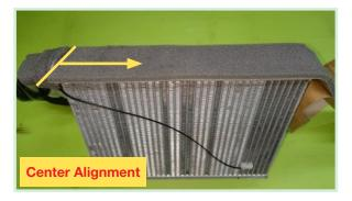
• Continue wrapping the insulation around the side surface of the evaporator while maintaining a center aligned installation.
