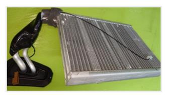
**IMPORTANT NOTE:** The connector insulation is overlapped by the evaporator core insulation. Use **CAUTION** when working in this area so the connection insulation is not damaged.
