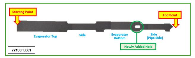
• Start from the connector insulation side of the evaporator top surface. Make sure the insulation is center aligned with the evaporator.
