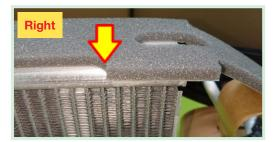
• Continue wrapping the insulation to the pipe side surface of the evaporator. Be sure to align the insulation centered onto the evaporator. Tuck the end portion of the insulation under the connector insulation as shown below.
