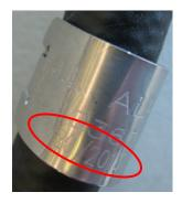
FIGURE 2-2. Motion Industries CNG hose metal ID tag includes date of manufacture (circled).
