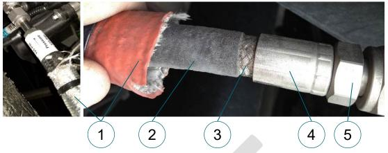
Figure 3–1. If hose is covered with a fire sleeve (1) or split loom, remove sleeve or loom to enable inspection of hose cover (2), braid (3), collet (4) and fitting (5).
