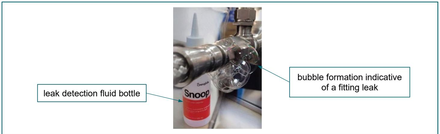
**FIGURE 4–3.** bubbles forming in leak detection fluid applied to a fitting junction
