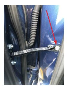
• Using the plastic trim tool, insert between the door frame and weatherstrip then twist it to release the 2 molded-in weatherstrip retaining clips as shown below. One clip is located at the top rear corner, the other in the top front corner.
