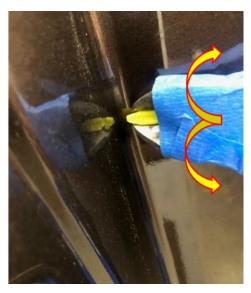
• As shown earlier, start in the upper front corner when installing the new weatherstrip. **REMINDER:** Make sure the 2 molded-in retaining clips are properly aligned with the square holes in the door frame **BEFORE** pressing them into place.
