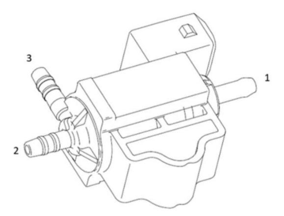
Note: Check port #2 to assure the spring gets lifted off the seat. This will be determined by the compressed air not dead-heading when applied to port #2. When applying air to this port a small amount of air should be observed at port #3 and even less air will be noticed at port #1. If this does not happen, the TCV plunger may have hardened deposits from hot operating conditions which will impede TCV plunger movement and the Turbocharger Wastegate Regulator Solenoid Valve should be replaced.
