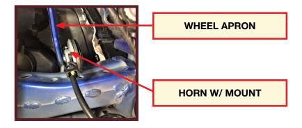
STEP 2) Slightly reposition the left horn mount towards the front of the vehicle. Use CAUTION not to apply excessive force causing damage to the mount. Function test the horn to in after adjustments to confirm there is no rattle/vibration sound during operation.
