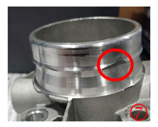
When the charge air cooler outlet tube has become disconnected from the throttle body, the tube end should be inspected for contact damage or a missing O-ring seal from blowing off.
