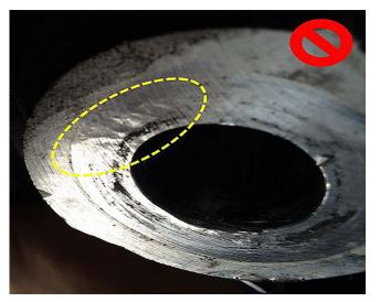
**4.7.** Next, visually inspect the knuckle's machined lower boss face, looking for evidence of material yielding. Yielding will manifest itself visually on this surface as a "bubbling" condition.
