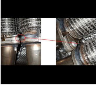
With a small punch or chisel and hammer bend/crimp the tabs on the exhaust gasket in further to prevent any spring-back and provide increased clearance between the two tabs to correct the noise or cutting the tabs off the gaskets is also acceptable.
