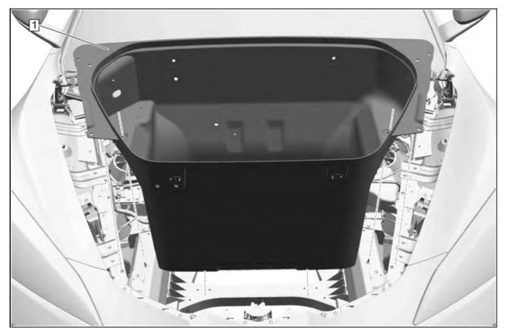
1. Remove the front compartment front panel (1). Refer to the appropriate *Front Compartment Front Panel Replacement* in SI.
