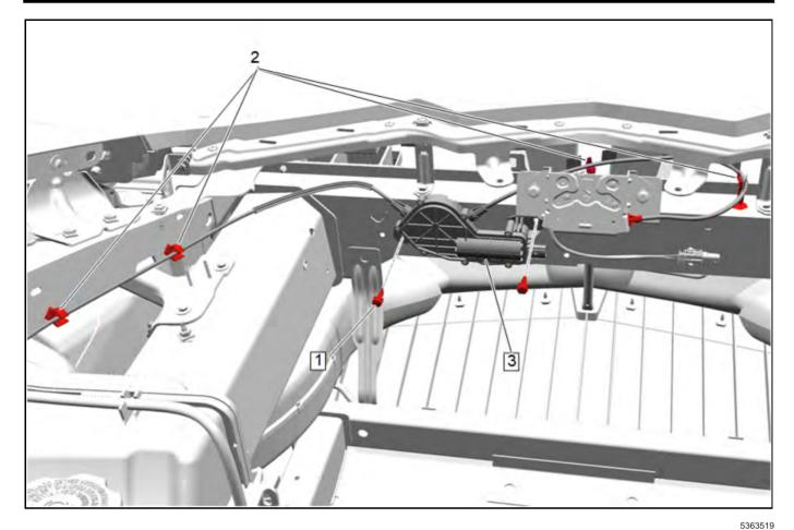
4. Remove the hood latch actuator. Refer to the appropriate *Hood Latch Actuator Replacement* in SI.
