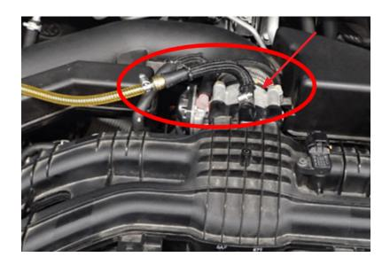
• STEP 7: Application of P.E.A. Carbon Cleaner into the Intake Manifold:
