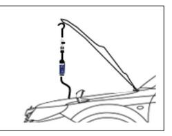
• **STEP 6:** Remove the purge hose located at the top of the throttle body as shown below and connect the hose from the applicator tool.
