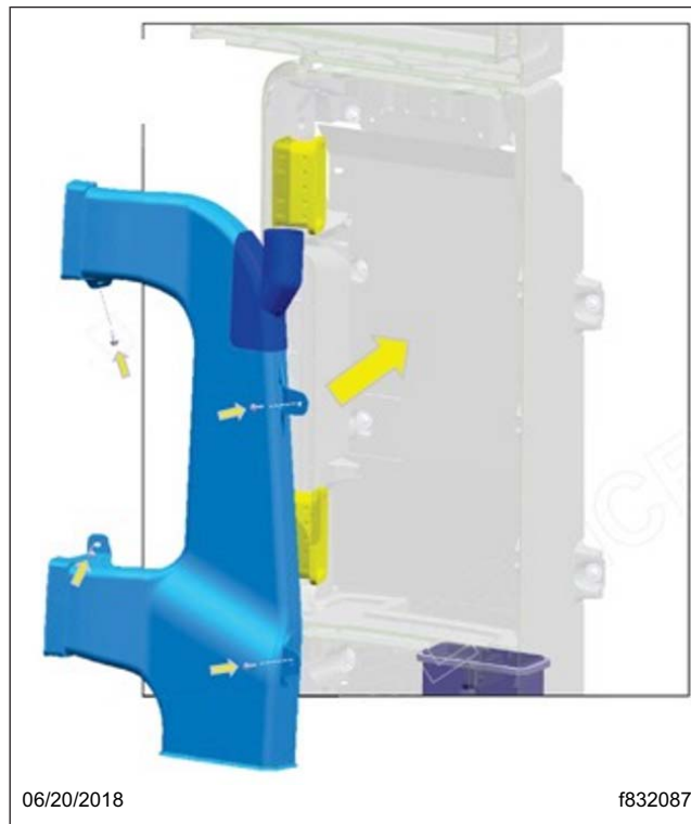
Fig. 9, Installing the Cabinet Ducting
