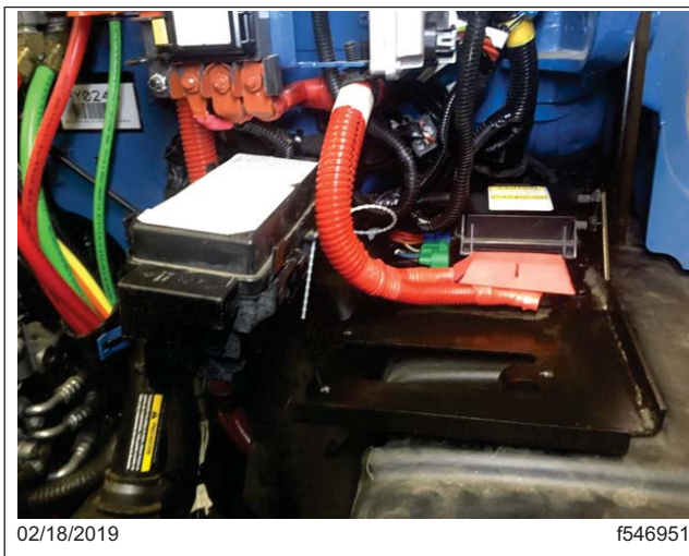
Fig. 6, Quarter Fender and PTPDM Installed on the Vehicle
