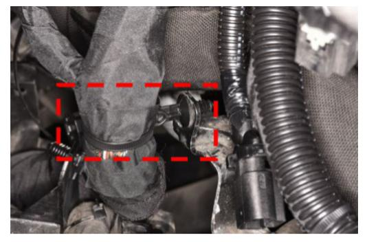
Protect the engine wiring harness from future damage at the top of the Camshaft Carrier Cover in the area shown below (1).
