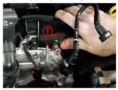
Inspect the engine harness at the Lower Air Cleaner Housing as shown below.
