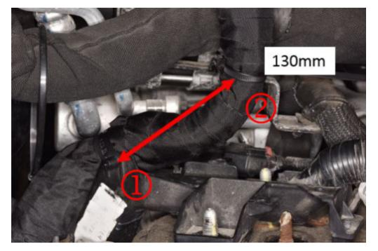
Measure up 155 mm from the Zip Tie style Fir Tree Clip located on the plastic Channel.
