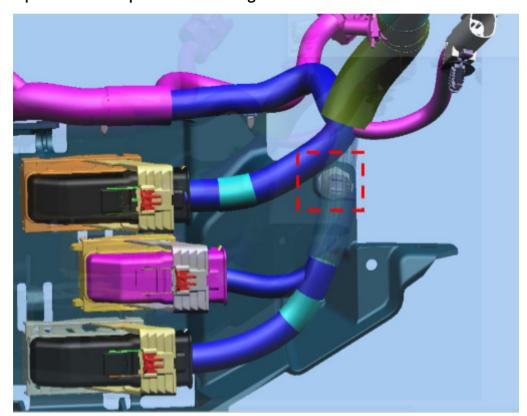
Protect the engine wiring harness from future damage at Generator Bracket.
