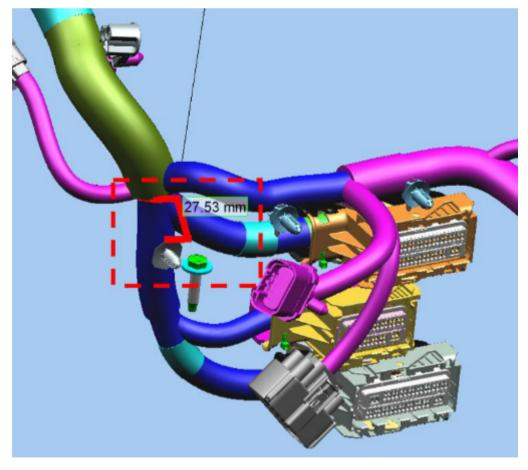
Insert the Zip Tie style Fir Tree Clip into the location shown below in the ECM Mounting Bracket.
