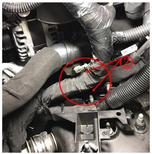
Inspect the engine harness at the Left Front Upper Control Arm Bushing as shown below.
