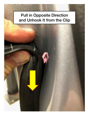
• Pull the rest of the weatherstrip from the channels at the top and upper back edges of the door.
