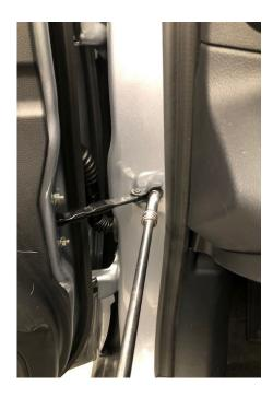
• Using the plastic trim tool, insert between the door frame and weatherstrip then twist it to release the 2 molded-in weatherstrip retaining clips as shown below. One clip is located at the top rear corner, the other in the front jamb area at the belt line.
