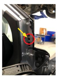
• Remove the original weatherstrip from the retaining T-clips securing it by CAREFULLY pulling the weatherstrip is one direction only enough to release it from one side of the "T" then unhooking it off the other side as shown in the sequence below. The replacement weatherstrips come with new T-Clips already installed.
