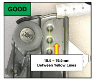
• In the NO GOOD photo above, the crimp tool edge has contacted the 3 "dimples" and the gap between them and the edge shown in the "GOOD" photos is exceeds 19.5mm. If EITHER of these conditions is identified, the window regulator assembly must be replaced.
