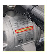
**IMPORTANT:** The NEW part <u>CANNOT</u> be identified by the Part Number. The production date code located on the compressor label must be used. In this example (**0087064586**), the "**0**" indicates the production year as 2020 (an "**9**" would be 2019, etc.). The next 2 digits, "**08**" indicate August as the production month ("**09**" would be September, etc.).
