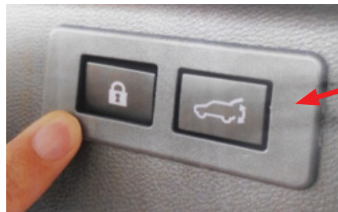
Here, the LOCK button is shown stuck below the surface of the switch trim cover.
