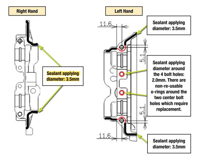
If you find engine oil seepage between the cylinder block and upper oil pan, remove the upper oil pan, clean the machined sealing surfaces thoroughly and then re-seal using Liquid Gasket ThreeBond 1217H (SOA868V9610) or equivalent\*. Note: The o-rings between the upper oil pan and the cylinder block along with those between the upper and lower oil pan will need to be replaced as they are not re-usable.
