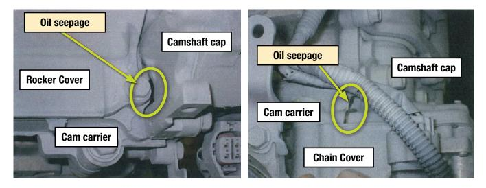
Apply Liquid Gasket, ThreeBond 1217H (SOA868V9610) or equivalent\* as shown below:
