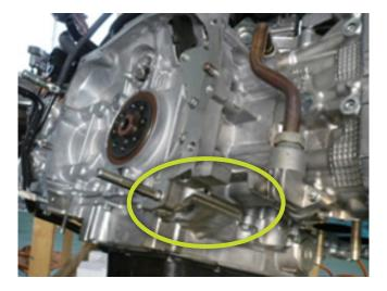
Photo shows seepage from upper oil pan to engine block sealing surfaces.
