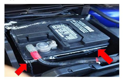
The RED arrows point to moisture seepage around the top cover seal and the start of an accumulation of corrosion. This photo depicts seepage which should be considered excessive and would be considered a warrantable defect requiring battery replacement.
