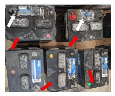
In this collection of returned batteries, the RED arrows point to moisture accumulations which has escaped from either the post seal(s) and / or the covers (fill caps) as a result of normal outgassing, a normal by-product of charging. The two WHITE arrows point to corrosion.
