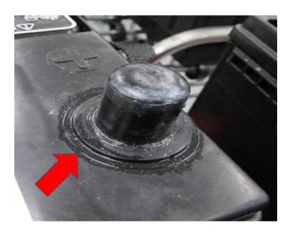
The RED arrow points to moisture seepage seen around the post seal. This photo depicts seepage which should be considered normal and would not be considered a warrantable defect requiring battery replacement.
