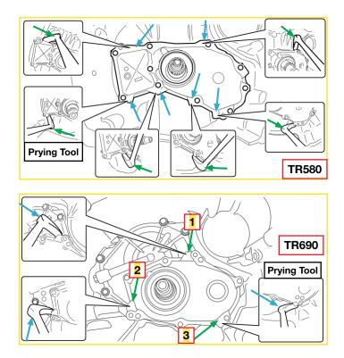
from the cover and mating surface of the housing. DO NOT use any abrasive or gasket removal / cleaning discs. Use the adhesive side of a piece of duct tape (or equivalent) to pick up any loose pieces of sealant material which may be found in the cavity around the stator support. DO NOT use compressed air.
