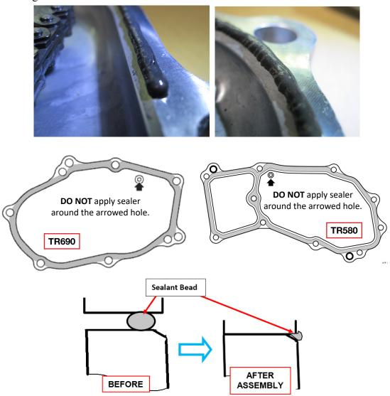
**NOTE:** As shown above, a properly applied, small bead of sealant will fill in the chamfered portion after the cover is installed. Do not use an excessive amount of sealant.
