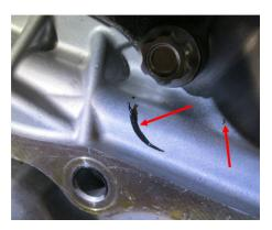
• Take note of how the sealant on the removed cover forms an additional "seal" when it becomes displaced into the chamfer around the inside edge of the case's machined surface
