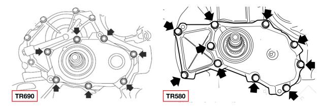
• Using a prying tool, CAREFULLY pry (GREEN arrows IN THE ORDER SHOWN for TR690 model) the cover loose from the housing. Pry ONLY on the specific areas or "tabs" of the pump cover indicated by the BLUE arrows. When the cover starts to come loose, continue to pry ONLY on the tabs and not the machined sealing surface of the cover.
