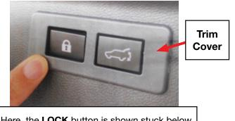
Here, the **LOCK** button is shown stuck below the surface of the switch trim cover.
