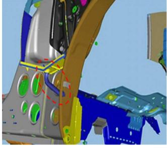
**Note:** The drain hose (shown circled above) runs from the quarter window cavity to the wheel well. A blockage or clog could occur at either end of the hose.
