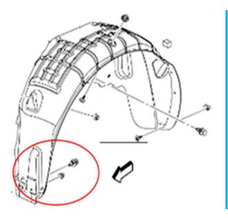
1. On the affected side of the vehicle, remove the forward, lower fasteners and pull back a portion of rear wheelhouse liner to gain access to the quarter drain dust flap (shown at the arrow). Refer to *Rear Wheelhouse Liner Replacement* in SI.
