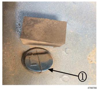
**Note:** Inspect for, and remove, any paint that may be holding the drain flap (1) shut.
