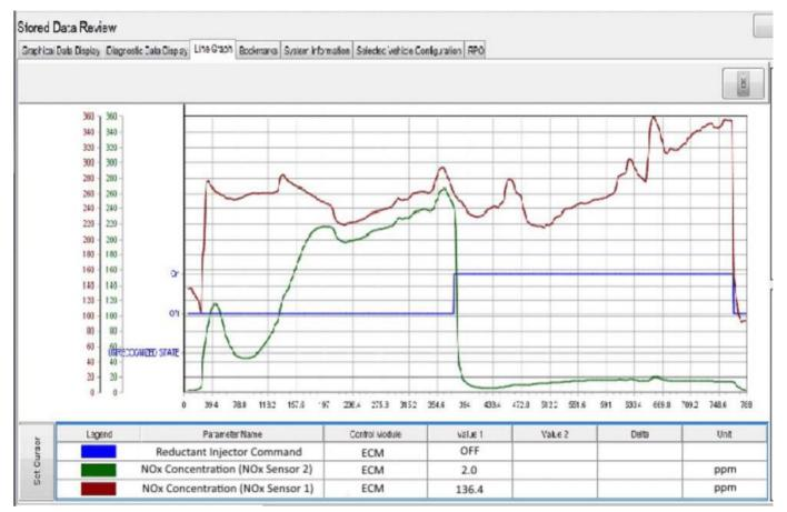
Graphed results of the NOx sensor readings during the a Reductant System Malfunction Warning Service Bay test.
