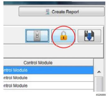
**Note:** The LOCK PARAMETER BUTTONS must be selected after each parameter has been selected to be graphed.
