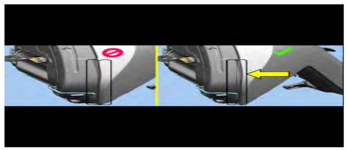
4.1. Start application of mylar tape by removing the liner from the narrower surface side.
