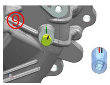
9) Remove the wrench socket and check the angles of parts marking.
