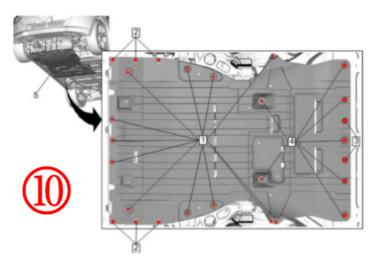
10) To gain access for inspection of plug 1 remove front compartment air deflector. (See also SI Service Document 4533740).
