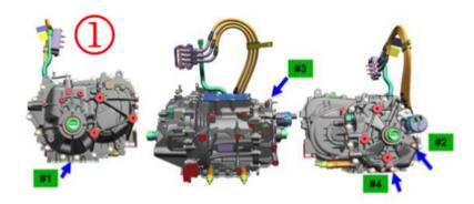
1) Purpose : Increase engagement of one thread pitch (4.5 - 5.5) and sealant (1-1.5 2-2.5pitch) by additional tightening (Rotation Angle : 380 - 400 degrees)
