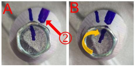
A) Inline Plug and cover for start point2) Limit band for final angle.
