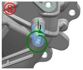
8) Tighten the plug 380-400 degrees (until red line meets cover marking.
