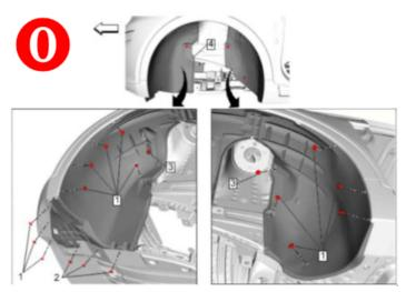
0) To gain access for inspection of plugs 2, 3 and 4 remove left front wheelhouse liner. (See also SI Service Document 4533734)
