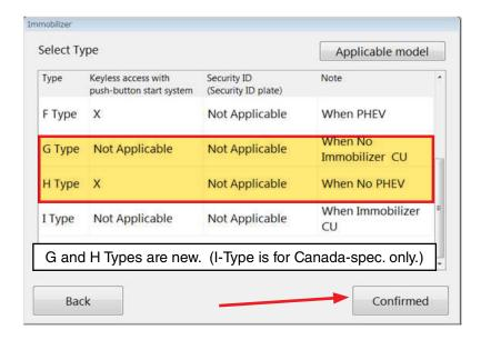
• When the vehicle utilizes either a **G** or **H** -Type system, an Authentication Key is required to perform any of the immobilizer-related functions listed in the menu shown below.
