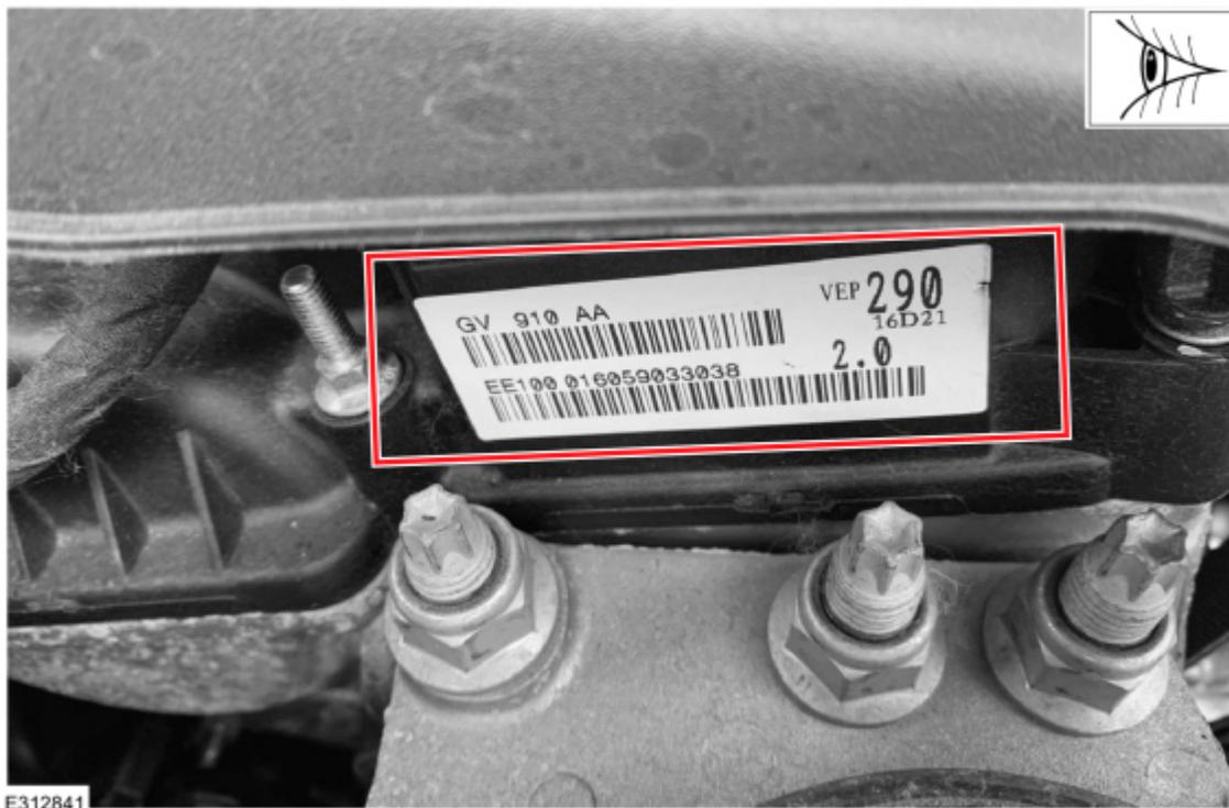
2. Does the engine base part number match the requirements listed in Step 1?
