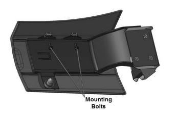
**4.** Install the complete DEF door assembly onto the front chassis fairing assembly by using the magnet locator to correctly position the door assembly.
