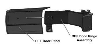
3. Install two (2) bolts (PN 996062) onto the spring nuts previously installed on DEF door panel.
