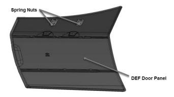
2. Slide and snap the DEF door hinge assembly (PN 84733141) into the snap features on backside of the DEF door panel (PN 84733671).
