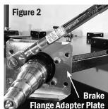
(blue) Loctite® 242 or equivalent on the threads and torque the bolts/nuts evenly in a star pattern to 35 ft. lbs..
