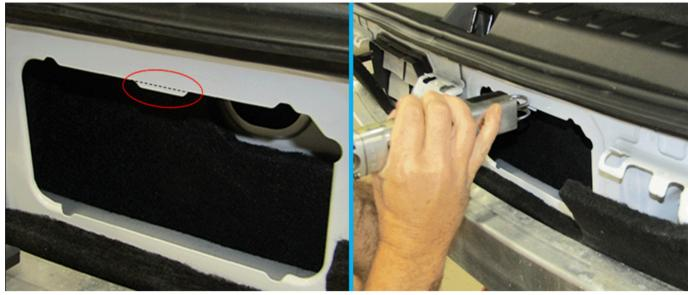
**Note:** The sheet metal tabs should be ground/cut off to be flush with the top edge of the opening.
