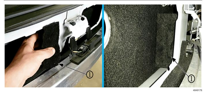
4. Install the acoustic insulator block (1) in the middle of the chamber, between both PRVs.
