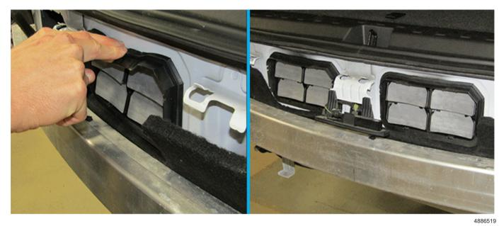
5.3. Seat the bottom of each PRV into the sheet metal opening, then snap into place at the top.
