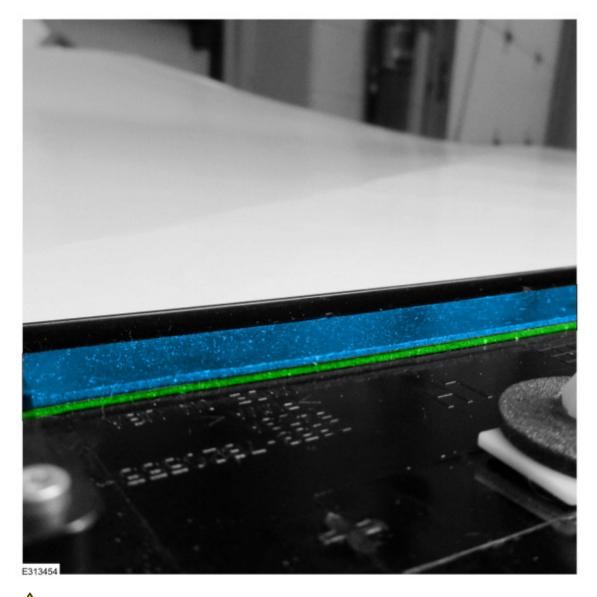
CAUTION: Do not allow isopropyl alcohol to contact the keyless entry keypad or rear door upper moulding to avoid damaging the plastic.
