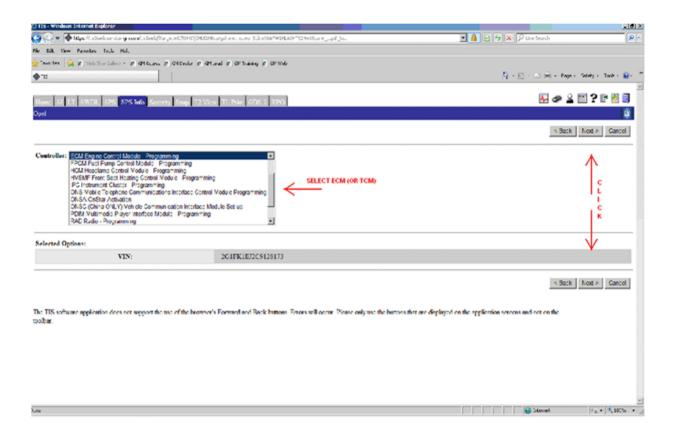
Select: ECM Engine Control Module — Programming from the Controller dropdown menu and select: Next.
