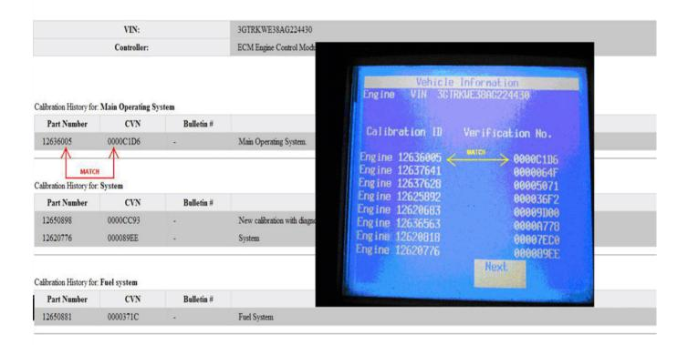
Compare each: Calibration ID Part Number and Verification No. (Number/CVN) from your Tech 2® photo to the corresponding Calibration ID Part Number and Verification No. (Number/CVN) listed in the TIS2WEB GM Vehicle Calibration Information screen of TIS2WEB to ensure that they are ALL an EXACT MATCH.
