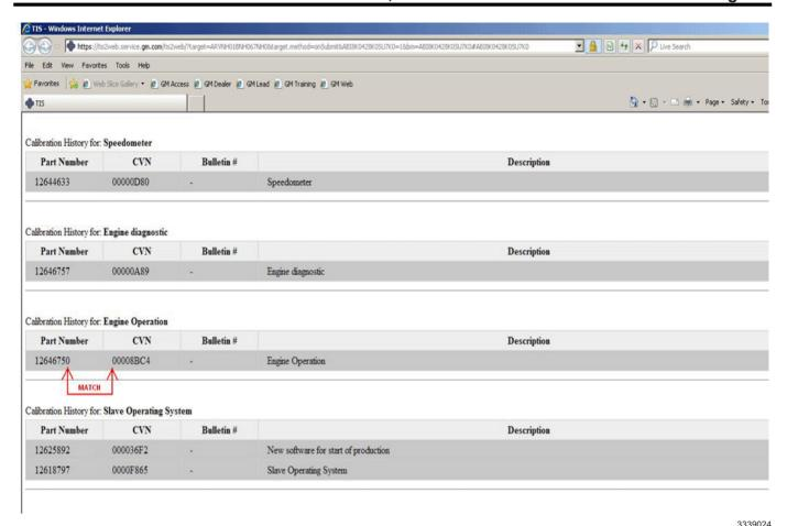
Compare each: Engine Calibration Part Number History parameter and Calibration Verification Number History parameter from the GDS 2 Calibration History screen to the Calibration Part Number and Calibration Verification Number (CVN) listed in the GM Vehicle Calibration Information screen of TIS2WEB to ensure that they are ALL an EXACT MATCH.
