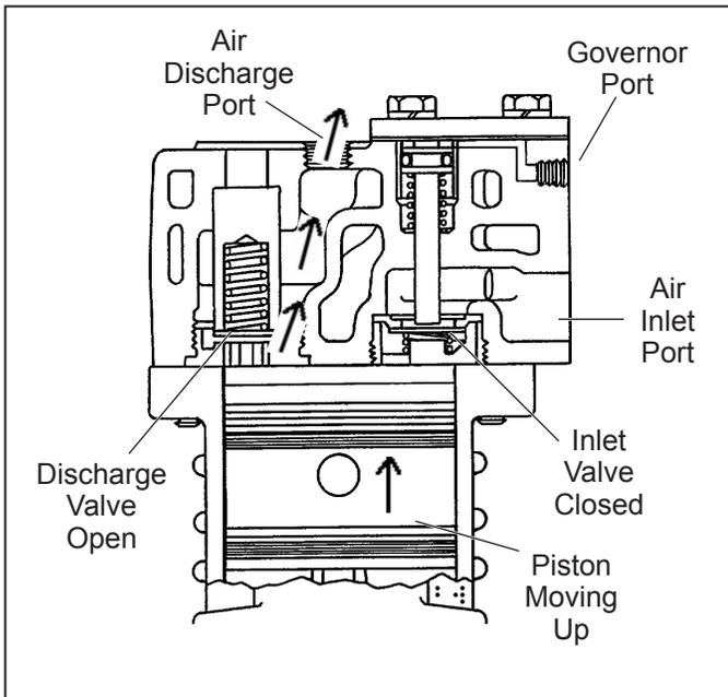
**Figure 6 – Operational-Loaded (Compression)**
