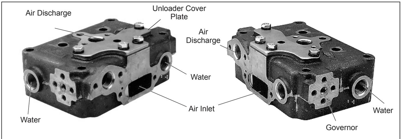
**Figure 2 – Cylinder Head**
