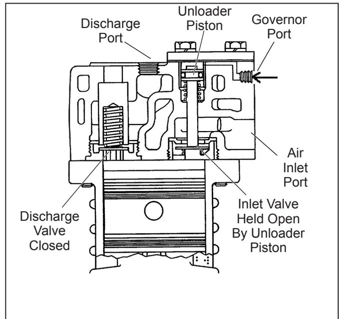
**Figure 7 – Operational-Unloaded**
