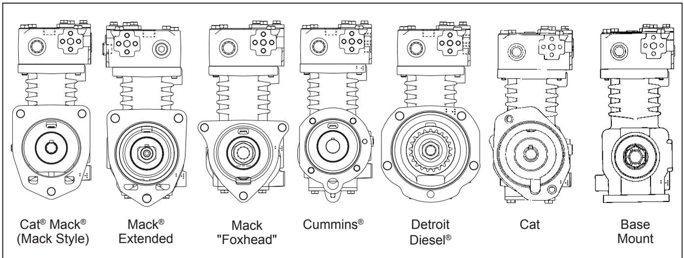
**Figure 3 – Flange Configurations**
