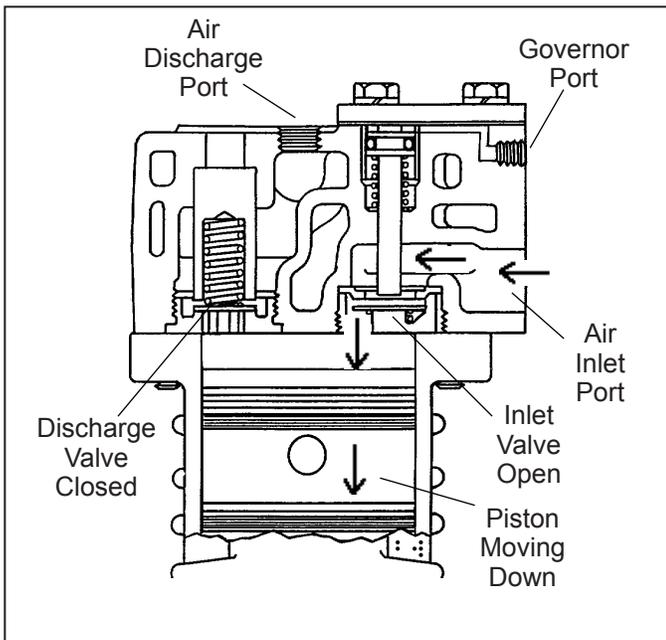
**Figure 5 – Operational-Loaded (Intake)**
