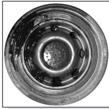
Oil shown leaking from an air dryer cartridge.
