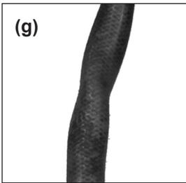
Partly collapsed inlet line shown.
