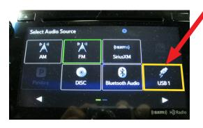
Install Drive "1" (or Drive "2" after successful installation of Drive "1" update is confirmed) into the vehicle's USB port. After the flash drive is recognized, the USB icon will illuminate.
