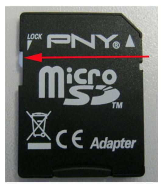
Note: While this system is capable of operating correctly with a micro SD card that has been inserted into a full sized SD card adapter, it has been found to work more reliably when a full size SD card used. Customers are strongly encouraged to use a standard size SD card with the PDR system in these vehicles.
