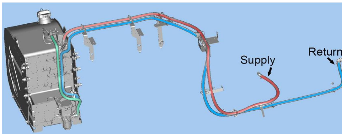
Figure 2: DEF Tank Coolant Line orientation for EPA 2017 vehicles
