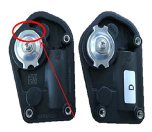
2. Use a vise to hold the actuator and cut off the leg, as shown in the illustration above, using a die grinder or cut-off wheel.
