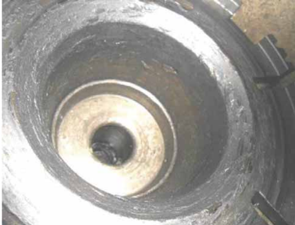
Spalled Bearing Race (Image 6)
