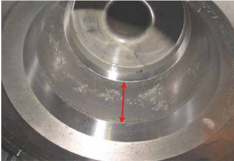
Spalled bearing race (Image 4)
