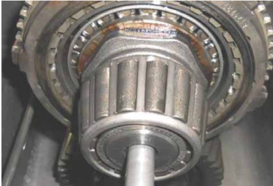
Spalled bearing failure (Image 3)
