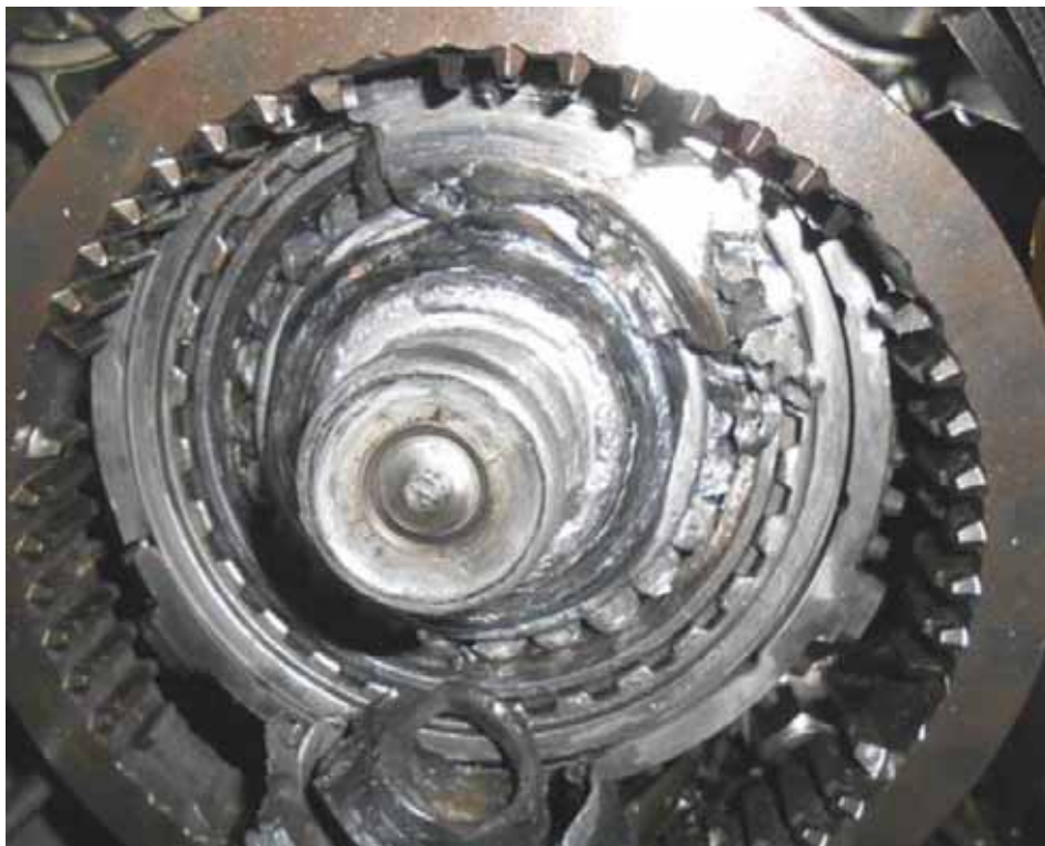
Spalled Bearing Failure (Image 5)
