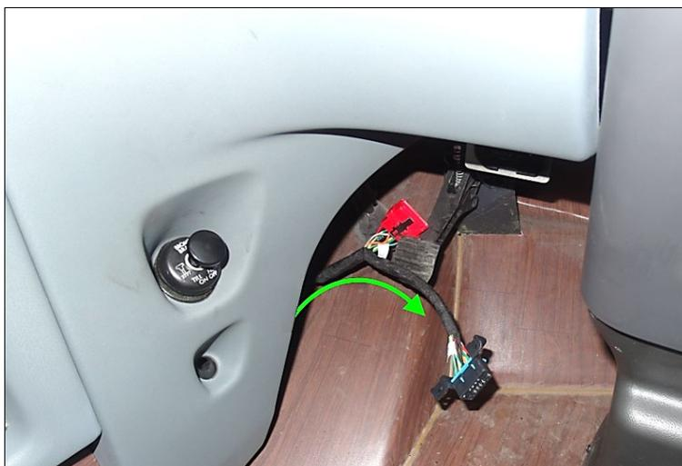
5. Connect the vehicle OBD connector (previously removed from the bracket) to the ELD harness red connector.
