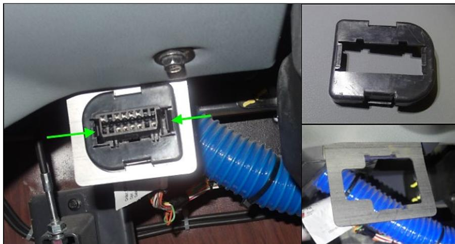
4. Route the ELD interface harness **23446648** from the electrical compartment up to the driver's area (OBD connector area).
