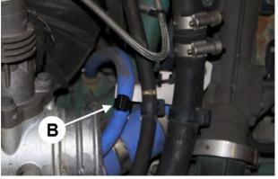
66. Hook up the "L.H. alternator power cable" #234524934 to the alternator positive (+) post. Place the flash washer between the cable lug and the nut.
