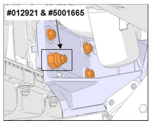
FIGURE 37 Tighten ground stud to 94 lb-ft Tighten stud nut to 94 lb-ft
