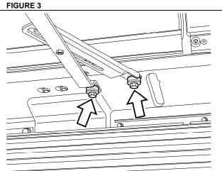
6. Remove radiator **sealing frame**.
