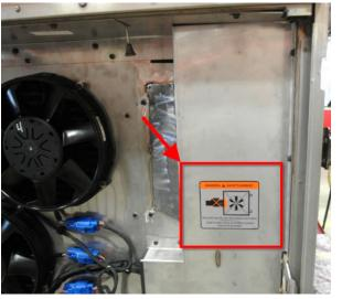
146. Install a second warning decal #069205 as shown on the radiator door.
