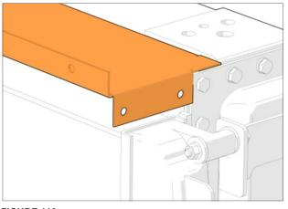
91. Install the sealing element #050203. Screw it on the existing threaded holes on the bottom of the radiator. Secure with the following hardware:
