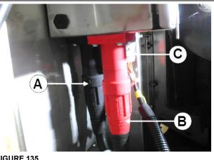
113. Secure the fan drive ground cable and the fan drive power cable connected to the fan drive circuit breakers box as shown on the pictures.
