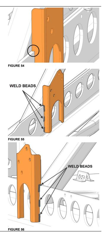
49. As a preparation to **welding**, buff the paint to reach bare metal. Weld the **ground stud** #380360 centered in the beam and at 14 inches from the beam end.
