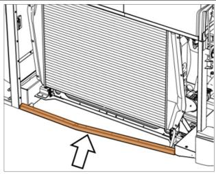
90. Install the sealing element #050200. Screw it on the existing threaded holes on the upper part of the radiator. Secure with the following hardware:
