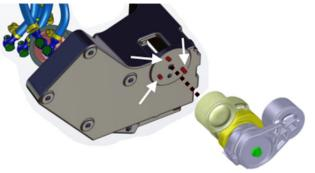
32. Reinstall the idler/tensioner assembly as a unit on the new L.H. engine mount #010090.
