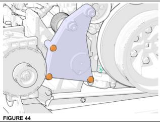
41. Install the new **idler #012349** with screw #5001786 and washer #5002008.
