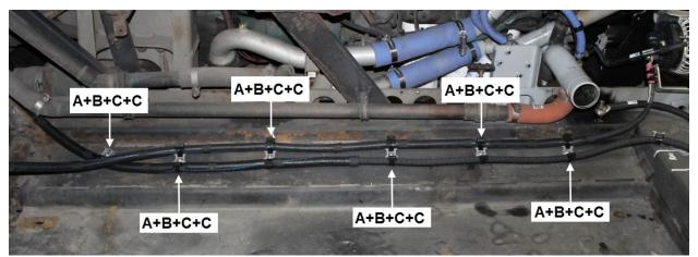
FIGURE 85 A: tie mount #509490 B: rivet #504610 C: nylon tie #509491
