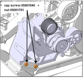
FIGURE 38 Tighten isolator screws to 60 lb-ft
