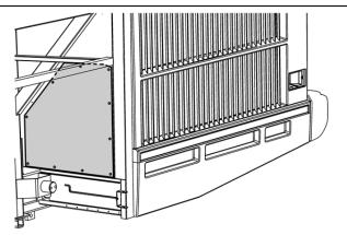
Open radiator door to access radiator assembly. Unfasten upper arm assembly.
