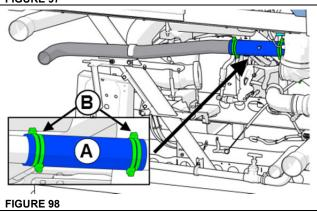
79. Install the new **CAC inlet pipe** #050286. Use one new #20550690 **CAC flexible hose**. Secure the hose using two (2) spring loaded clamps #21490630.
