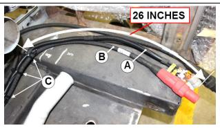
FIGURE 89 A: FAN TO RJB INTERFACE" HARNESS #23488790 B: FAN DRIVE POWER CABLE C: NYLON TIES #504016 (23x approx.)
