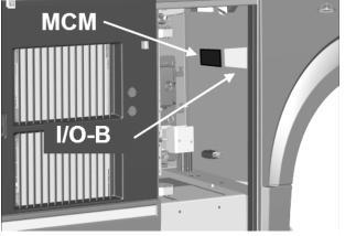
FIGURE 151: MAIN POWER COMPARTMENT
