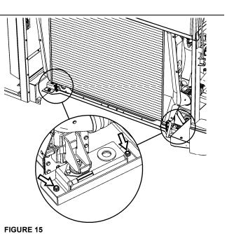
18. Position a **forklift** under the radiator assembly that is capable of safely lifting the radiator. With assistance, slide radiator assembly out and onto the forklift. Transfer radiator assembly to a secure location.
