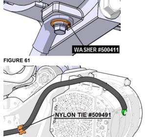
54. Secure the alternator ground cable to the previously installed ground stud on the L.H. engine mount.
