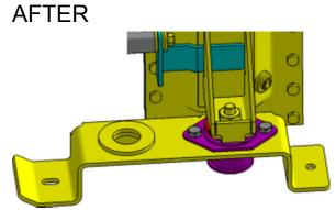
FIGURE 21: MOUNTING SUPPORT AFTER 180° ROTATION
