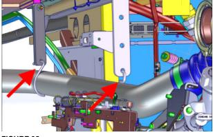
76. If your vehicle is equipped with AFSS (Automatic Fire Suppression System), the new CAC outlet pipe #050406 is likely to come into interference with a AFSS extinguishing agent hose (see image) near the end of the pipe that connects with the Charge Air Cooler.
