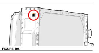
85. Install the brass fitting assembly in place of the former vent hose fitting and then connect the radiator vent hose to the radiator.
