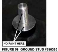
52. Install the alternator ground cable #0610035. Use the ground screw and lock washer supplied with alternator with the addition of a flat washer #500411.
