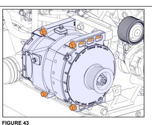
40. Install the idler support #011213 using: *3x screws* #5001799
