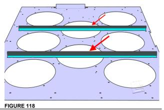
96. Install the fan support panel **#050195**. Secure with the following hardware:
