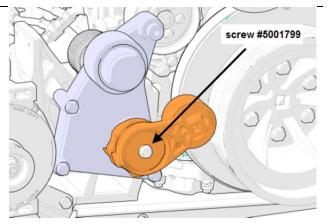
FIGURE 48: Tensioner mounting screw torque : 48 lb-ft
