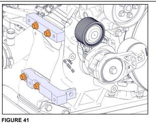
38. Installing the LH alternator pulley. Place #560720 alternator flat on a bench with the shaft horizontal.
