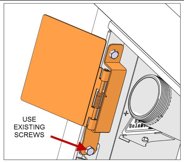
FIGURE 2: X3 MODELS WITH LOCK MODELS FLAP INSTALLATION
