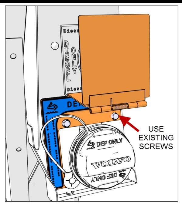
FIGURE 1: H3 MODELS FLAP INSTALLATION
