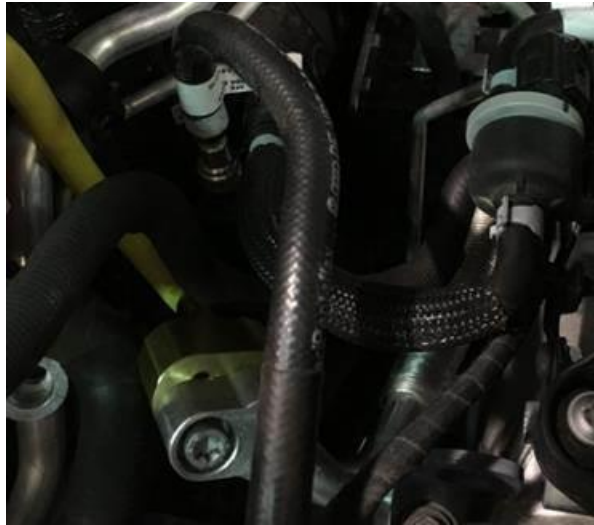
Figure 15. Attaching service station and flush hoses to rear A/C lines.
