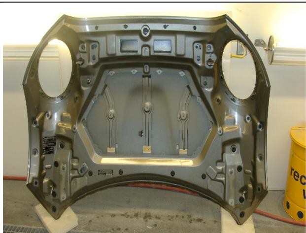
9. If body panel hanger is not available, the hood can be rested in the position shown. Use foam blocks as shown to prevent damage to the corners and surface of the hood.
