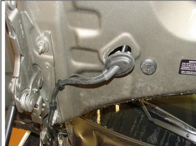
7. Feed washer hose out of hood before hood removal.
