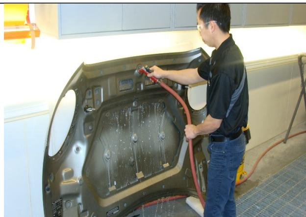
12. After 15 minutes has elapsed, rinse out all cavities and underside of the hood with water starting from the top down. If possible, use **lukewarm** (not hot) water for a more effective removal of the wax.
