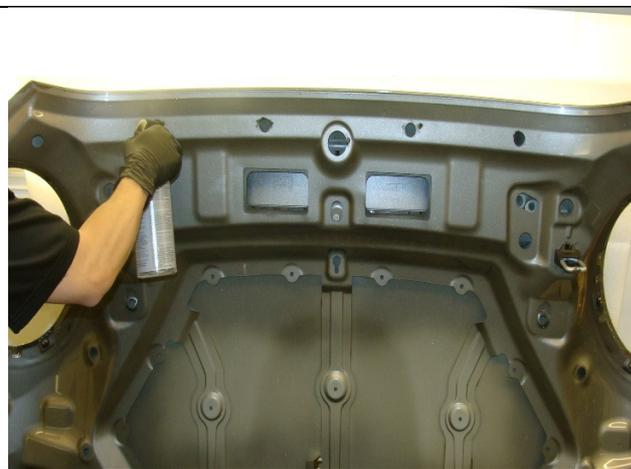
11. Once the plugs are removed, apply the cavity wax **remover** liberally to all of the cavities starting from the top down. Use  $\frac{1}{2}$  of the bottle, the other  $\frac{1}{2}$  is to be used for the second application.
