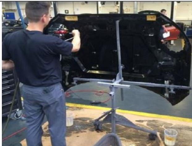
8. Remove hood completely from the vehicle and place into body panel hanger, or:
