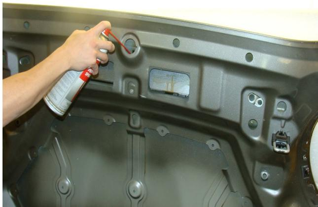
15. Once the hood has been thoroughly rinsed and dried, re-apply cavity wax to cavities in the hood. Start from the top and work down spraying a small amount into all holes and cavities.
