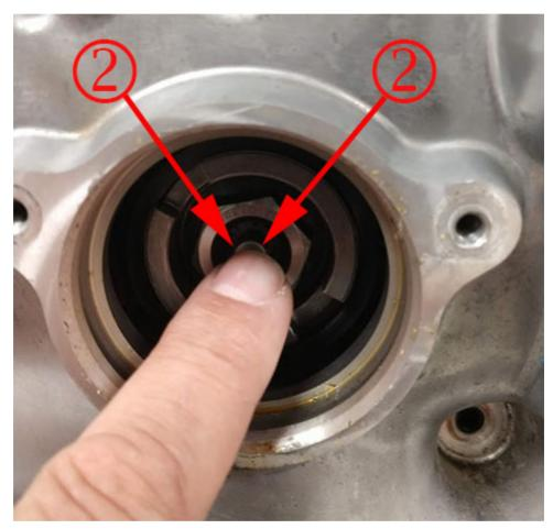
If the spring is broken, the plunger travel may be decreased, it may not fully return to the proud position, and may have poor spring tension as compared to a new assembly.
