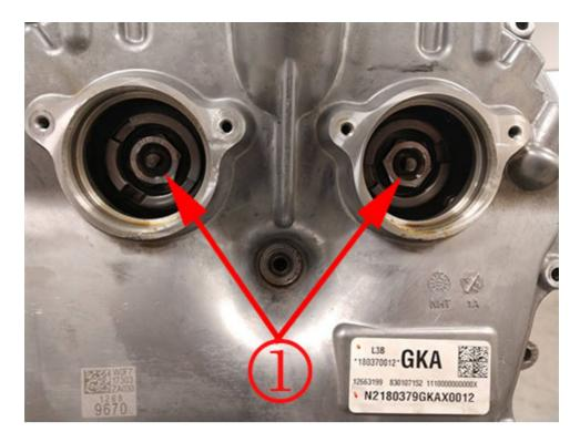
Using your finger, compare the travel and feel of the Camshaft Position Actuator Valve Bolt Plungers (2) to each other.
