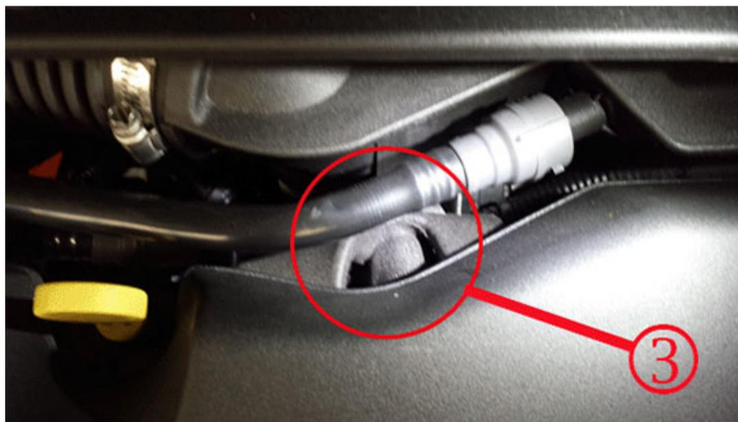
**3) Foam installed folded over, contacting the line**
