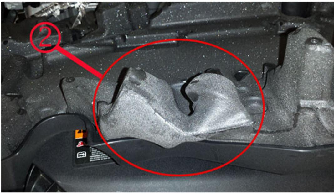
**2) Foam is Deformed from heat**
