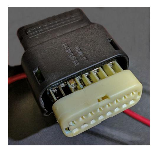
If water intrusion or corrosion is found replace all affected terminals on the body side with terminated leads and replace the rear fascia wiring harness.
