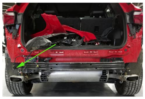
If no obvious terminal concerns are found it may be necessary to remove the TPA to be able to view inside the connector for moisture.
